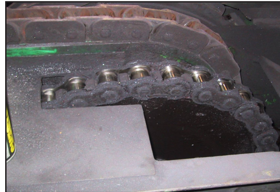
Heavy scale and surface contamination prevented re-lubrication by normal oils.
